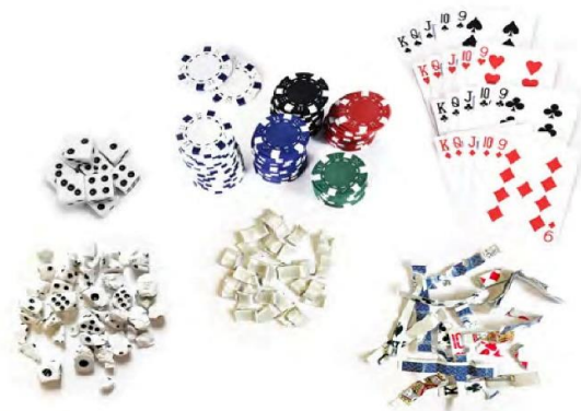
Shredded material samples: 12,5 x 20 mm dices and plastic chips shreds 12,5 x 20-88 mm playing cards shreds
